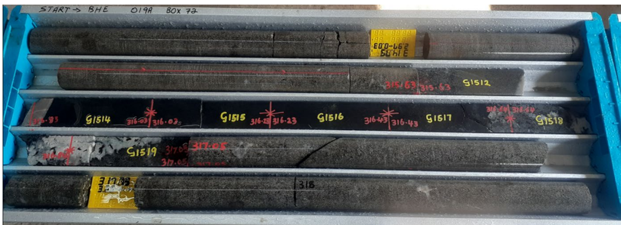
Figure 1. A 76cm interval of the UG2 Reef in hole E019a after sampling
