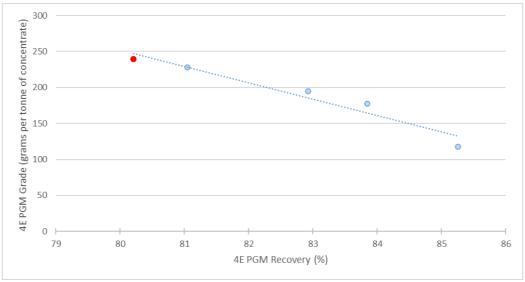
Figure 6: Concentrate grade vs. recovery (4E)
