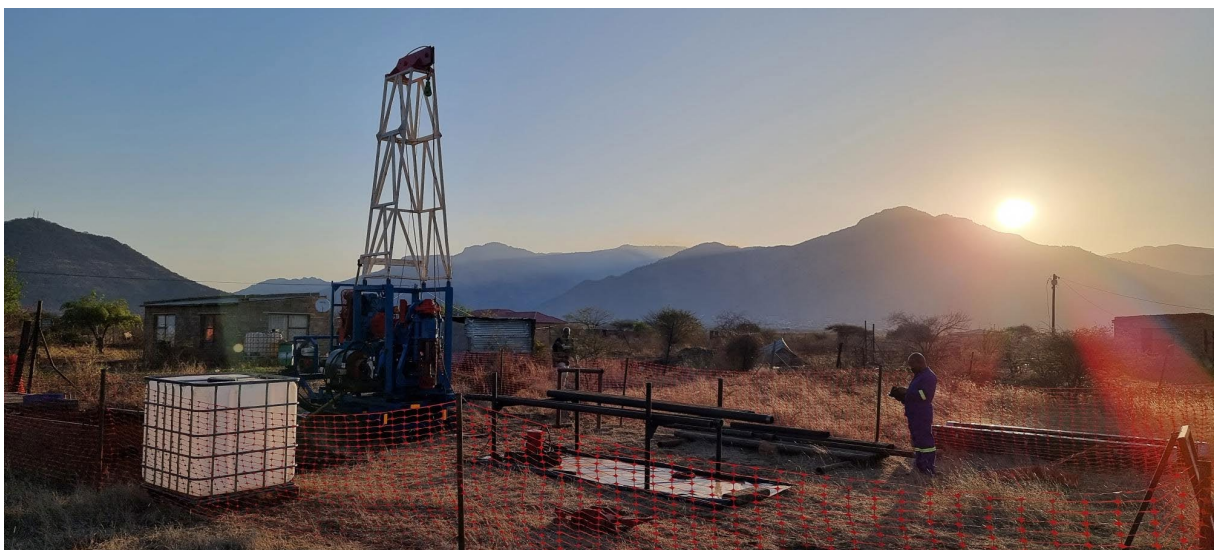
Figure 2: YWE D90R drill rig set up at drill site E060 ready to commence drilling in the next day or two
