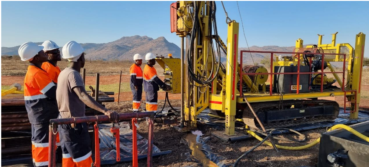
Figure 5: Drill team and geological workers deploy the Atlas Copco CS-1500 drill at Bengwenyama
