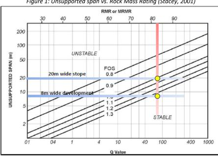
Figure 1: Unsupported span vs. Rock Mass Rating (Stacey, 2001)
