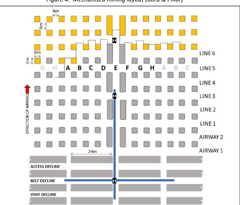
Figure 4: Mechanised mining layout (Bord & Pillar)
